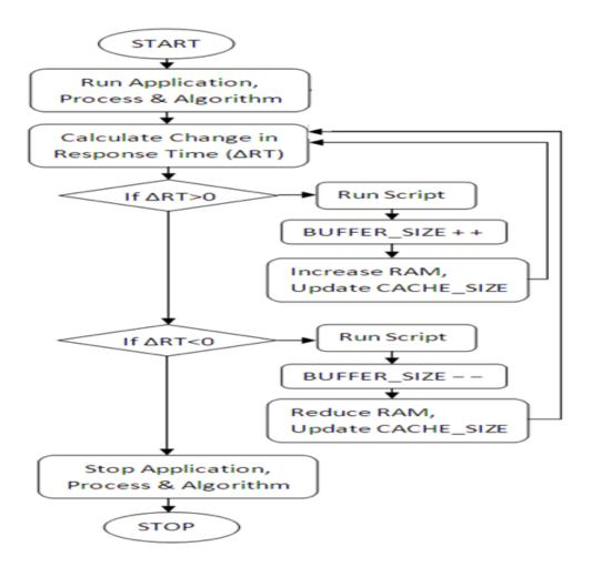
Fig.5. Flowchart for Automated Tuning
