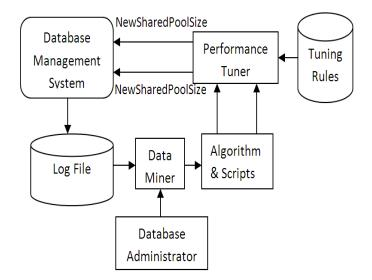
Fig.3. Script based Tuning architecture
