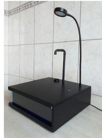
**Fig. 6.** SmartGarden – water and light sources
